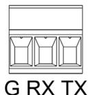
Parameters (DIP switch 2 selectable): 9600 baud, No parity, 8 data bits, 1 stop bit **or**
