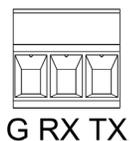
Parameters (DIP Switch 2 OFF): 9600 baud, No parity, 8 data bits, 1 stop bit
